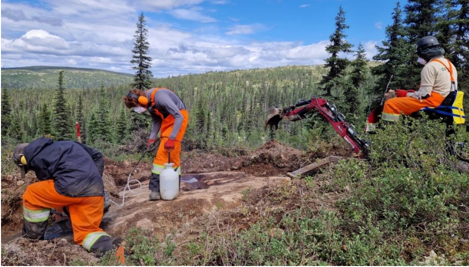
Fig. 2: Stelmine workers stripping outcrop with the mini-excavator and carrying out channel sampling in the new sector.
