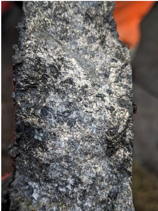
Fig. 3 : Typical rock from the first channel sample of the new area. The mafic host rock shows semi-massive patches of pyrrhotite, locally with interstitial chalcopyrite and traces of arsenopyrite.
